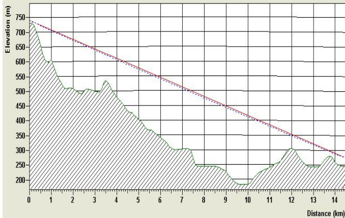
Fig.5 Terrain cut of link D → B
