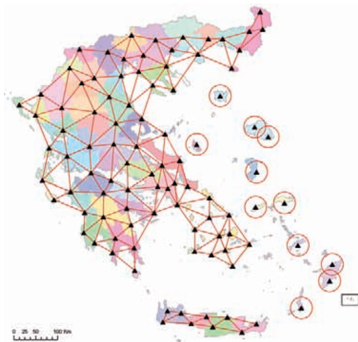
Figure 1: The established HEPOS network consisting of 98 reference stations.
