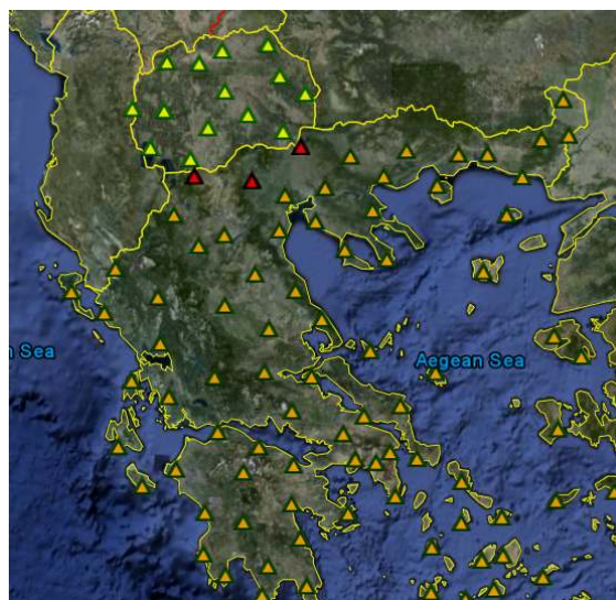
Fig. 4 The three HEPOS stations (in red) used for the connection between Greece and FYROM.
