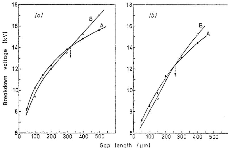
Figure 1. Breakdown voltage versus gap length for degassed oil. Sphere electrode: (a) etched; (b) anodized. A, point positive; B, point negative.
