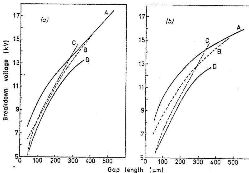
**Figure 4.** Breakdown voltage versus gap length for (a) a negative point, (b) a positive point. A, degassed oil, sphere etched; B, degassed oil, sphere anodized; C, oil saturated with oxygen, sphere etched; D, oil saturated with oxygen, sphere anodized.
