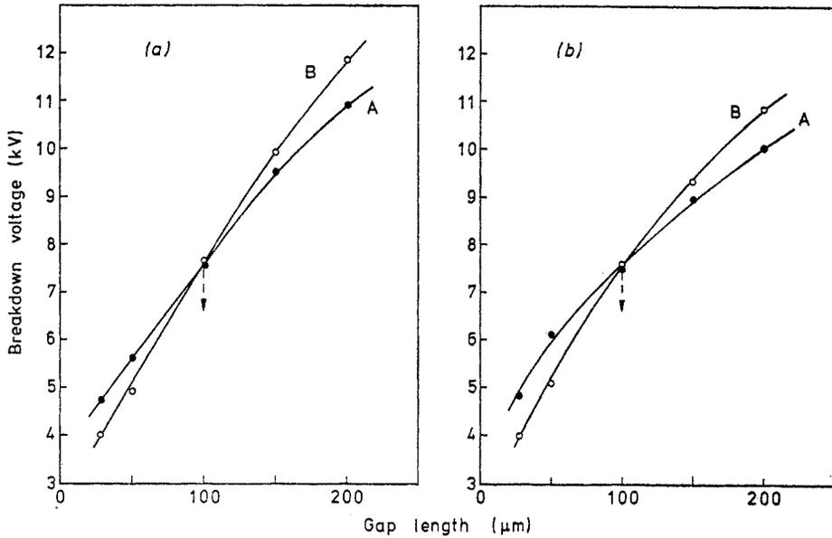
Figure 3. Breakdown voltage versus gap length for oil saturated with nitrogen. Sphere electrode: (a) etched; (b) anodized. A, point positive; B, point negative.
