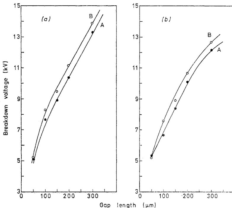
Figure 2. Breakdown voltage versus gap length for oil saturated with oxygen. Sphere electrode: (a) etched; (b) anodized. A, point positive; B, point negative.
