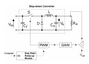
Fig.6. Step-down converter
