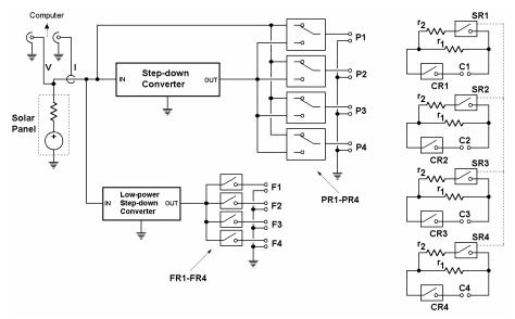
Fig.5. Schematic representation of the control system.
