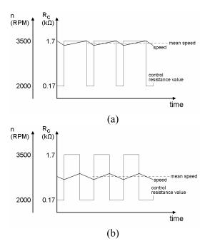
Fig.3. Hysteretic control of the compressor speed.
