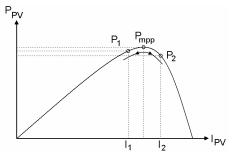
Fig.4. Maximum power traking.
