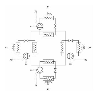
Fig.2. Schematic representation of the refrigeration system.
