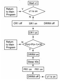
Fig.9. Compressor speed control pattern.
