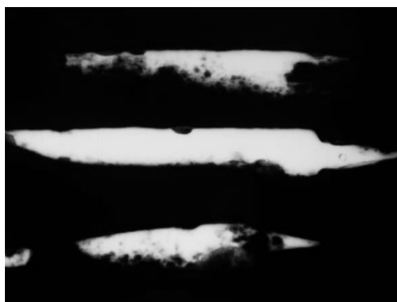
Photo 29: X-Radiography (55kV, 10mAs, 1sec) White areas indicate presence of metal core, grey areas indicate corrosion products and black areas absence of metal.
