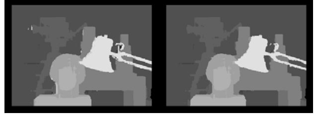
Figure 5. Disparity map of the left Tsukuba image before (left) and after (right) occlusions and mismatches have been handled.
