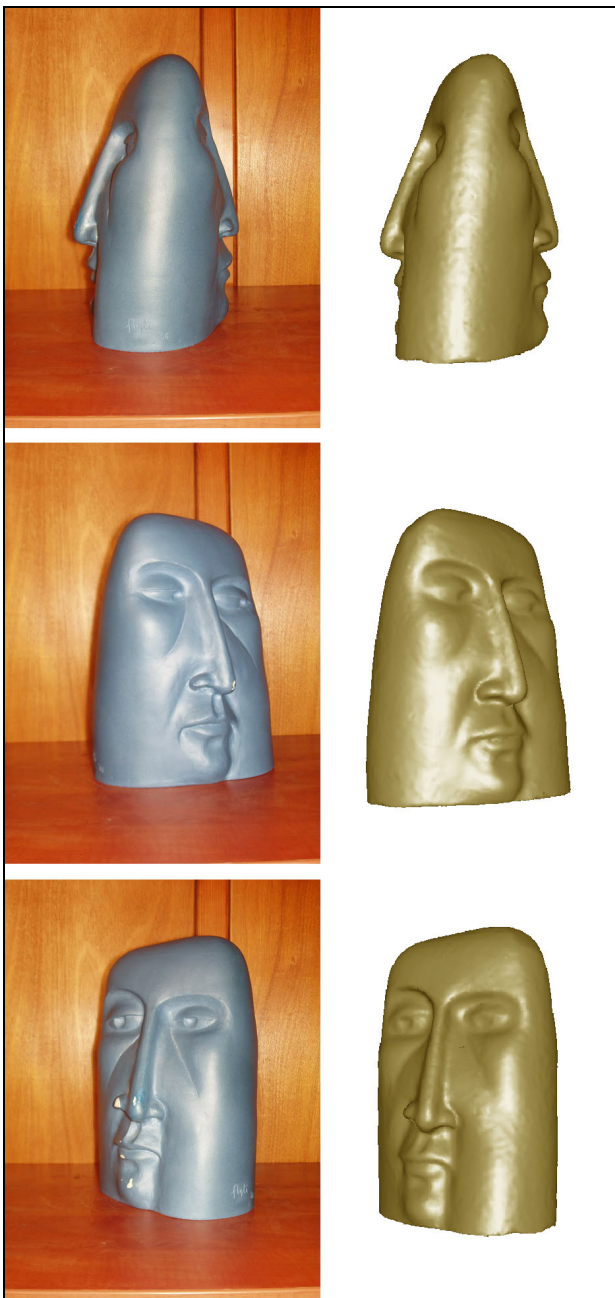
Figure 9. Different views of the object (left) and corresponding views of the rendered 3D model (right).
