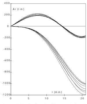
Figure 3. Initial and calibrated radial symmetric distortion curves for the RMC Tokina lens.
