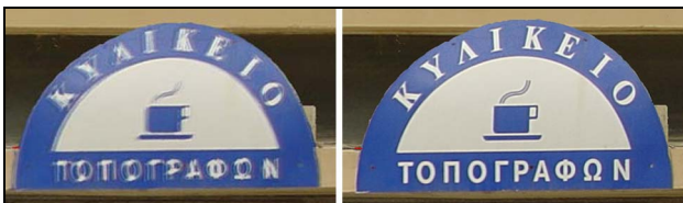
Figure 7. Orthoimage details from 7 images without (left) and with correction of radial lens distortion (right).
