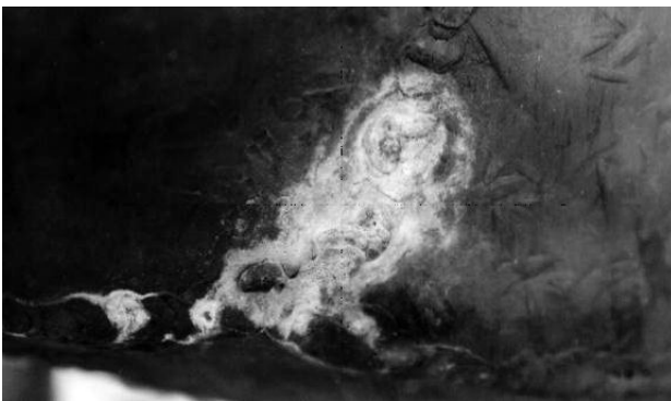
Fig. 10: Layer of green corrosion products.
