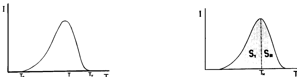
Fig. 1. The shaded area in the ITC band is proportional to the polarization decay P(T) .
