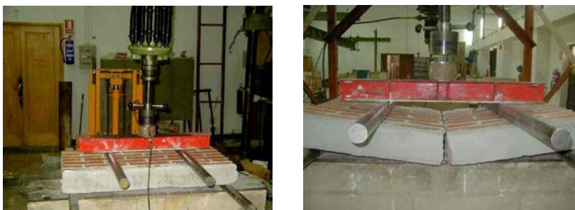
Figure 4. Failure perpendicular to bed joints.
