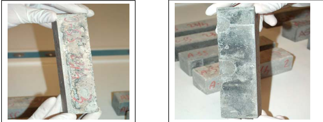
Figure 4. CM specimen (left) and SLM one (right) after 340-day to exposure to the leachate solution.
