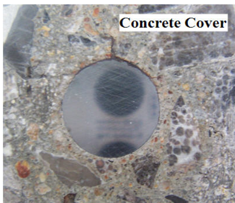
Figure 6 Corrosion distributions under artificial climate environment
