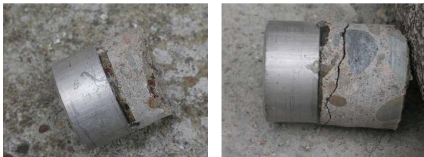
Figure 17-18: Two extracted cores of the pull-off test wich show different positions of the plans of separation.
