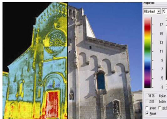
Figure 2. The thermographic survey on Cathedral's façade
