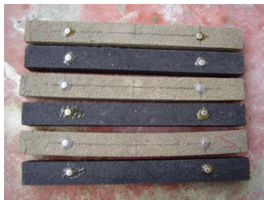
Figure 5. OPC specimen expand more than POFA specimen.
