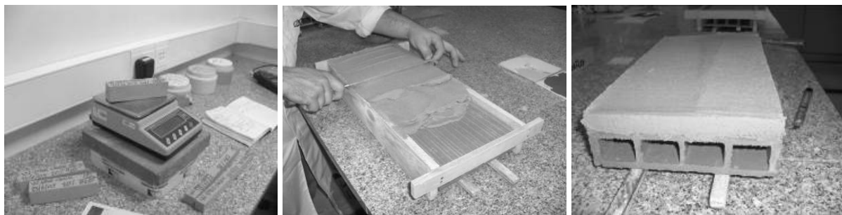
Figure 2. Standard prisms of rendering mortar (left), and small-scale models (centre and right).
