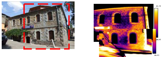
Figure 6. The infrared image of the selected region at the north façade, showing the severe material loss as warmer areas and the detachments which were not observed visually as colder areas, both suffering from the roof drainage faults [Disli et al. June 2007], [Disli et al. September 2007].
