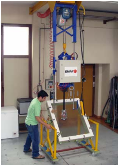
Figure 4. Test apparatus and tilted steel frame with mounting for a wood framed window glass
