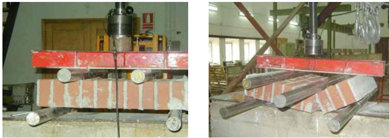
Figure 3. Failure parallel to bed joints.
