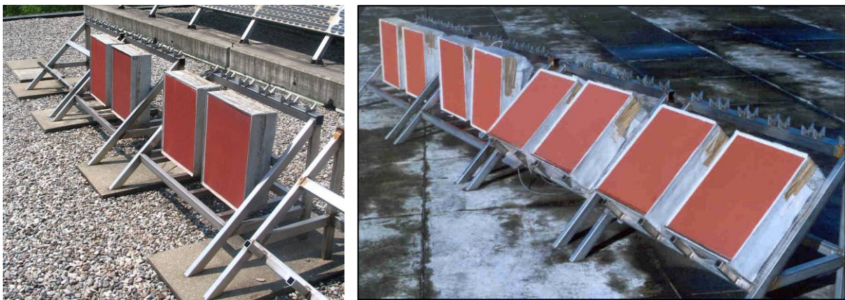
Figure 1. Natural ageing asset in Lugano (picture on the left) and Milano (picture on the right). The comparative analysis between the two contexts is related most of all to the pollution level, and to temperatures and radiation levels.
