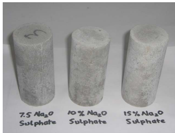
Figure 5. Geopolymer mortars with different Na 2 O to FA ratio after 12 weeks of immersion
