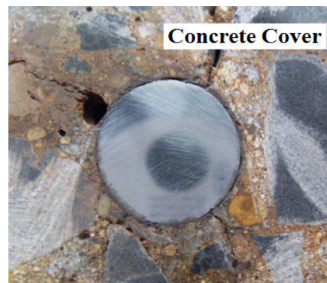
Figure 7 Corrosion distributions using the Galvanostatic method
