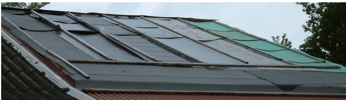
Figure 1. Test set-up for exposure to natural climate. The 7 roof underlays were placed on a south-facing roof with a pitch of 20°.
