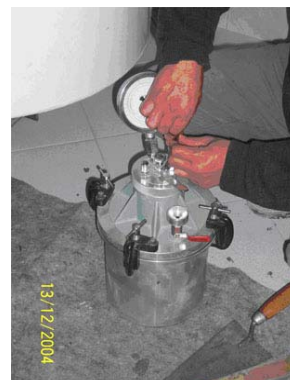
Figure 6. Determining the air content in the concrete mix with pressurized vessel testing.
