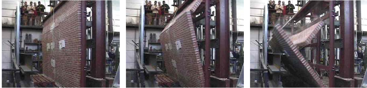
Figure 6. Bending failure sequence for a 3 x 5-m wall.
