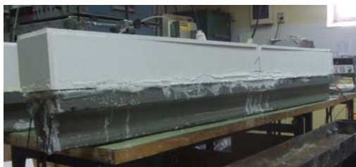
Figure 1. Prestressed T beam dimensions, with a pool fixed at the surface containing 0.5M NaCl (left) and connections for accelerated Cl penetration test (right).
