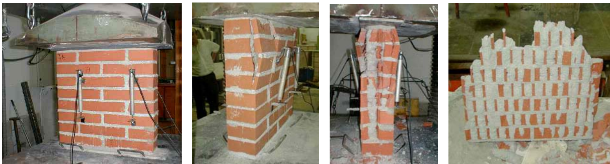
Figure 2. Test specimen before and after compression failure.
