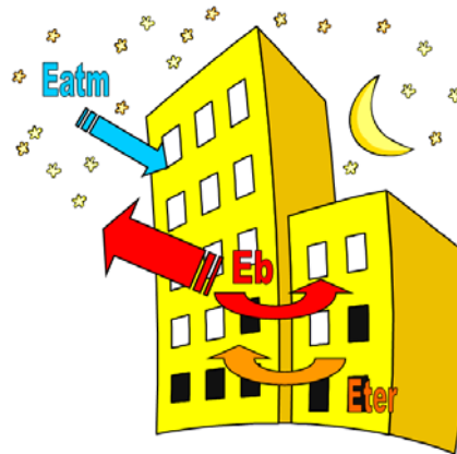
Figure 3. Radiant balance of a building's façade.
