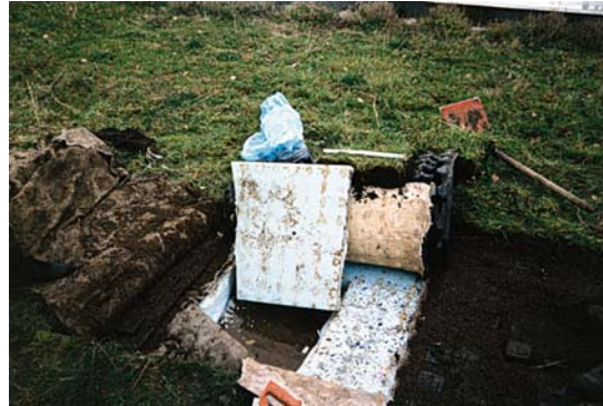
Figure 6. Sampling of XPS boards from a green roof (Photo: Dow Building Solutions).
