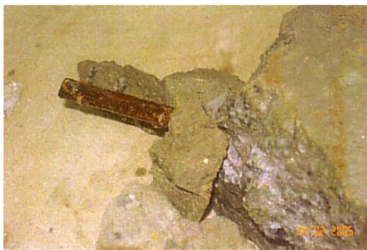
Figure 9. Condition of reinforcement in 40% NaCl solution after 45 days exposure period.
