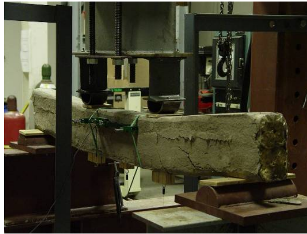
Figure 2. The bending test set up for a small scale OSCC beam.
