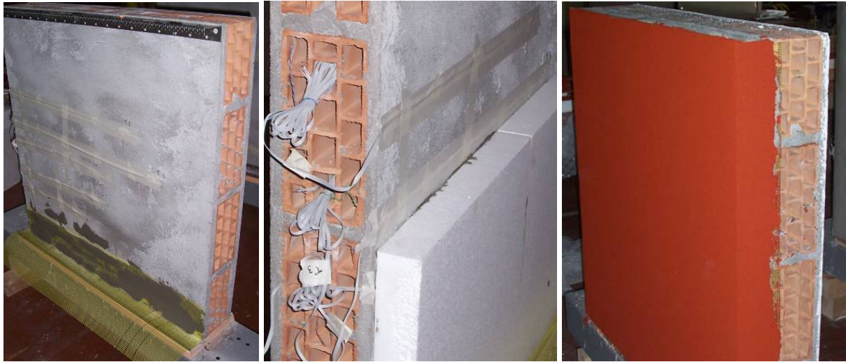
Figure 1. Sample A.1, Base coat with vinyl additive and finishing coat with acrylic resin.
