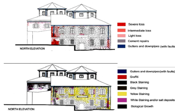
Figure 5. The maps showing the distribution of material loss (at top) and the distribution of discoloration and deposits on surfaces of the north façade (at bottom). The severe loss and detachment on surfaces was observed together with white staining and salt deposits, especially at the lower parts of the rainwater pipes at both sides of the façade and stone courses at the top, underneath the eaves gutter[Disli et al. June 2007].
