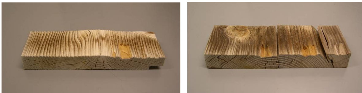
Figure 1. Photos of wood sample A (left) and wood sample H (right) after 115 days of accelerated ageing in the Atlas Solar Simulator climate chamber. Direct solar radiation exposed side shown upwards. Small wood pieces are cut from the samples for use in the FTIR investigations.
