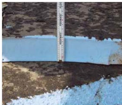
Figure7. Cross section of XPS insulation board after more than 20 years of service in an Inverted Roof outside of the water-proofing layer (Photo: Dow Building Solutions).
