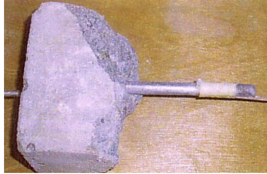
Figure 7. Condition of reinforcement in controlled sample after 45 days exposure period.
