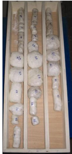
Figure 4. The samples have been wrapped up in the plastic film, covered with paraffin
