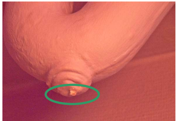
Figure 6. The result of lacking watertightness of the extended floor gully is seen as a drop on the water lock (inside the marking) in the flat underneath after flooding the floor above under 10 mm water for about 10 minutes.
