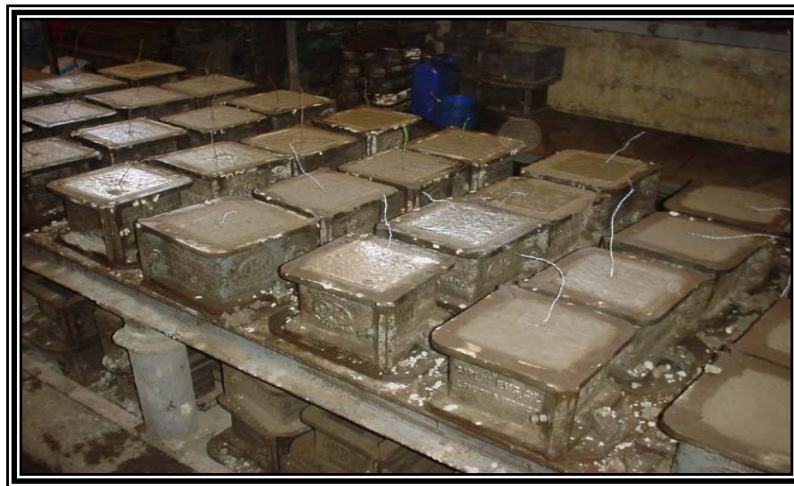
Figure 2. Thermocouples Sensors Installed in Specimens.
