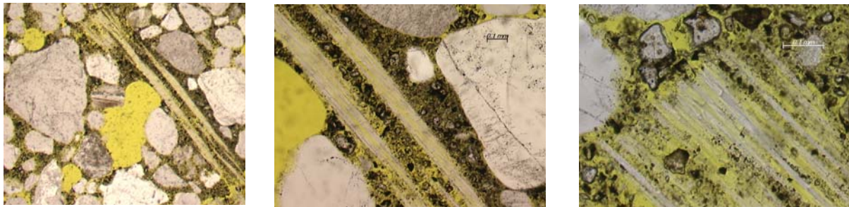
Figure 3.1. a, and b the bio fibers, and c, glass fibers for comparison
