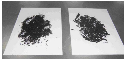
Figure 1. Short and long rubber fibres (RRF1 and RRF4) obtained by shredding discarded tyres.
