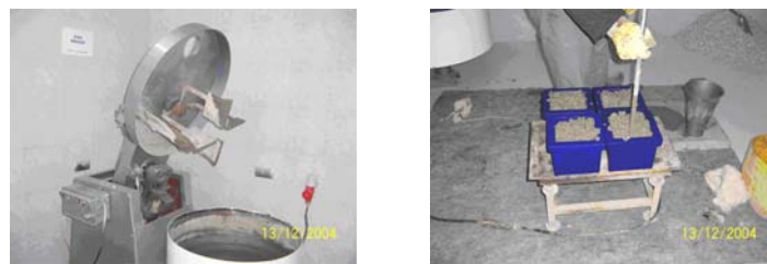
Figure 3. Mixing the concrete in the pan-mixer and Preparing test-samples by compacting concrete mix into moulds placed on the vibration table.
