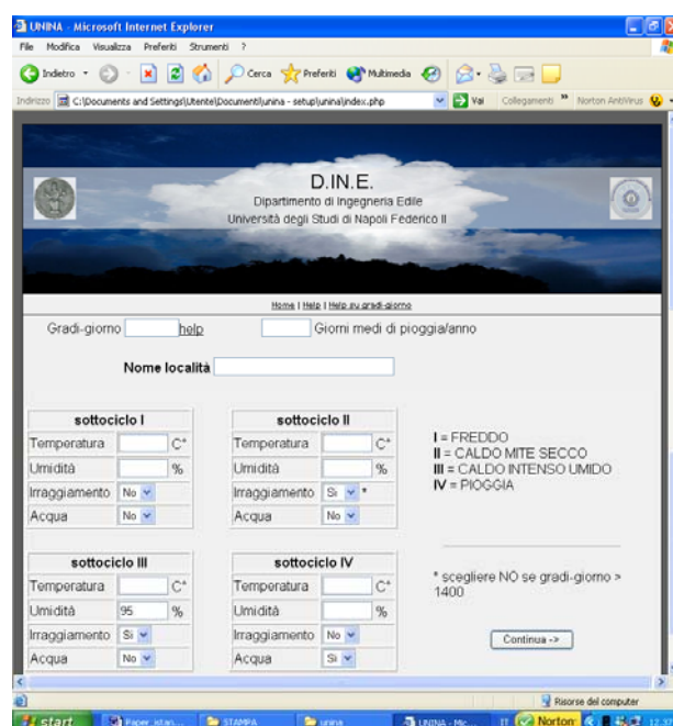
Figure 3. A screen from the software for the automatic composition of accelerated ageing sub-cycles in any climatic context.
