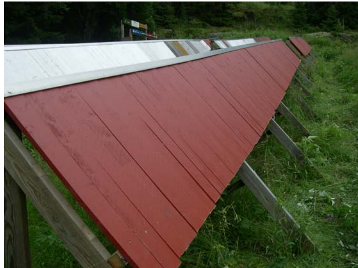
Figure 2. Wood cladding specimens mounted at the outdoor test site at Sørkedalen, Oslo.
