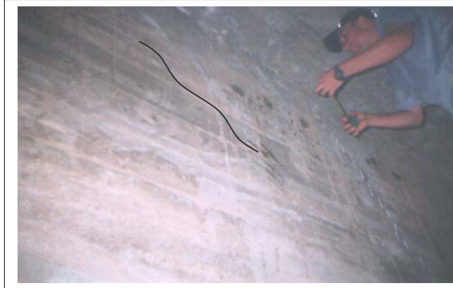
Figure 4. Ultrasonic assessment of cracks repair
