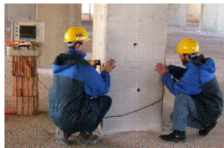
Figure 2. In situ ultrasonic test
