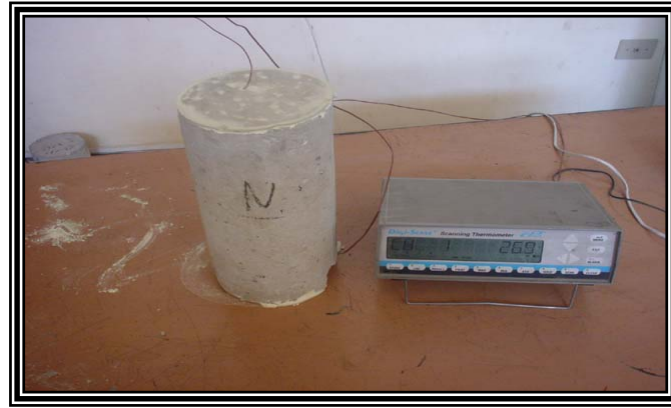
Figure 1. A device to Monitor and Record Concrete Temperatures.
