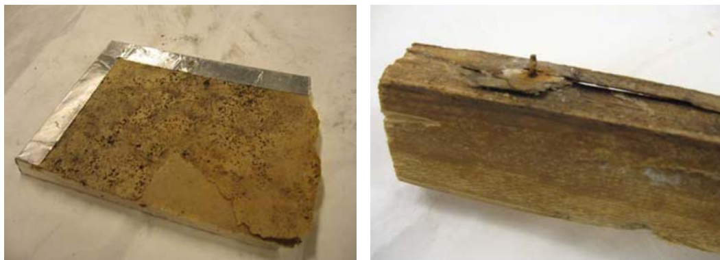
Figure 1. Photos of the large field samples from where smaller samples have been collected for the FTIR measurements. Mould fungi on GU plaster board (left photo) and mould fungi on wood and wood rot (right photo). GU = exterior grade gypsum board ("outdoor use").
