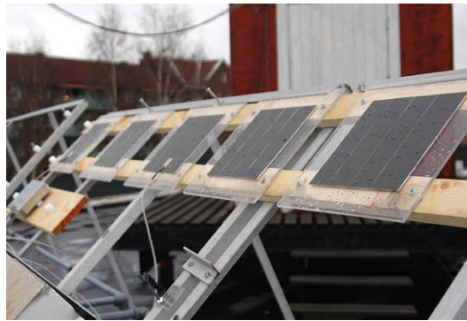
Figure 2. The natural field exposure set-up of the USC optical durability test. 5 test panels mounted onto a rack facing south and having an incline of 45^{\circ} .
