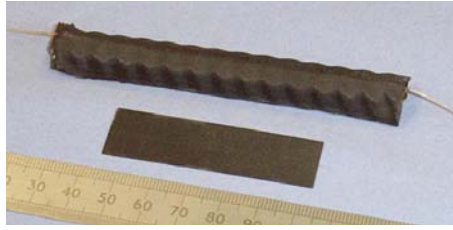
Figure 1. Optic fibres protected by carbon fibre cladding to be embedded into reinforced concrete and composite structures
