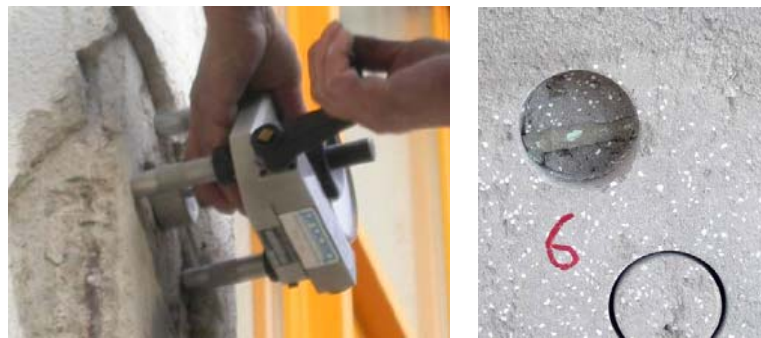
Figure 15-16. Determination of bond strenght by pull-off test.
