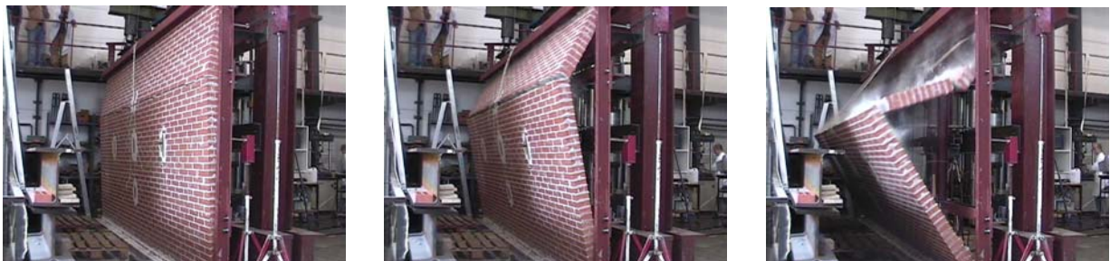
Figures 10 to 12. Failure sequence, 5 x 2.5-m wall.
