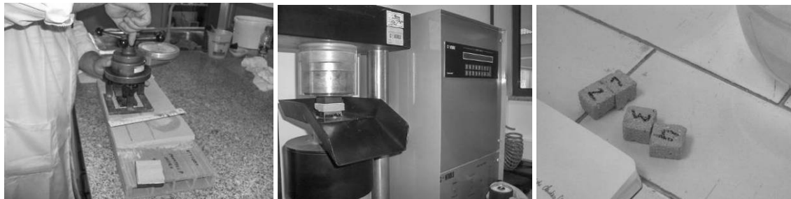
Figure 3. Pull-off test (left), compressive strength test with small samples (centre), and samples for open porosity determination (right).
