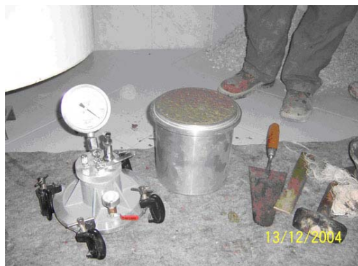
Figure 6. Determining the air content in the concrete mix with pressurized vessel testing.
