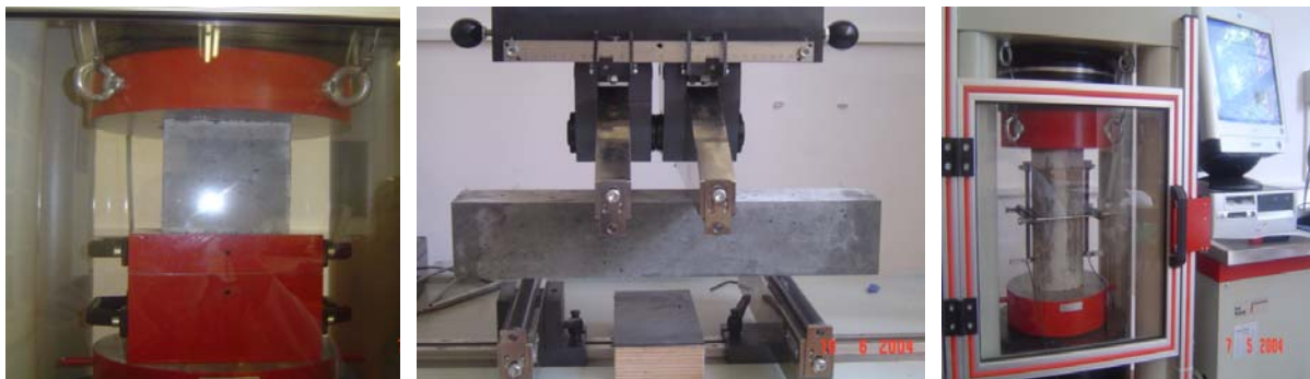
Figure 1. Concrete mechanical properties tests required to numerically model compressive strength (left), flexural strength (middle), and modulus of elasticity (right).
