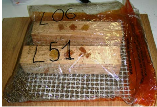
Figure 3. Inoculated stakes (44 x 44 x 200 mm)
