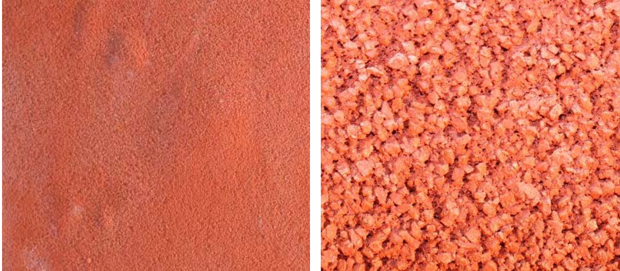
Figure 6. (Left side) Photograph of ETICS finish coat at ageing time T1; blisters (larger ones: 10 cm diameter circa) are evident on the surface of the sample; (Right-side) dimension of pores and surface appearance are changed (aggregate dimension 0/1 mm); Localized fading due to rain-wash is shown.
