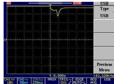
Fig.9 PV voltage waveform during startup of the compressor with the proposed controller. Scales: 10V/div, 250ms/div.
